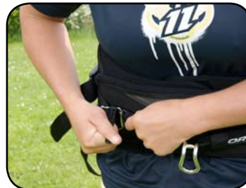
Push release tab down and out away from you, while pushing quick-release clip button.
