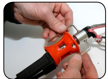
Using both allen keys, tighten pin and screw simultaneously in opposing directions.
