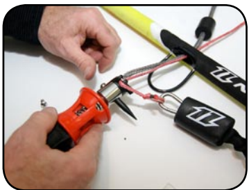
Pin and threading tool pushed all the way through hole.
