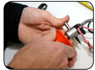
Once pin has caught loop inside, push pin all the way through.
