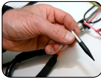
This will be used to thread the Depower Line knot into the Iron Heart.
