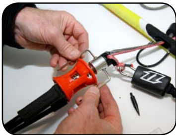
Use allen keys to unscrew screw and pin simultaneously in opposite directions.
