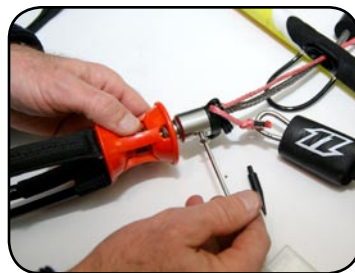
Using allen key, insert screw.
