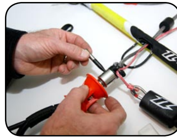
Push through hole from one side of Iron Heart, making sure you catch the loop inside.
