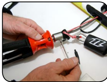
Pull out pin and screw.
